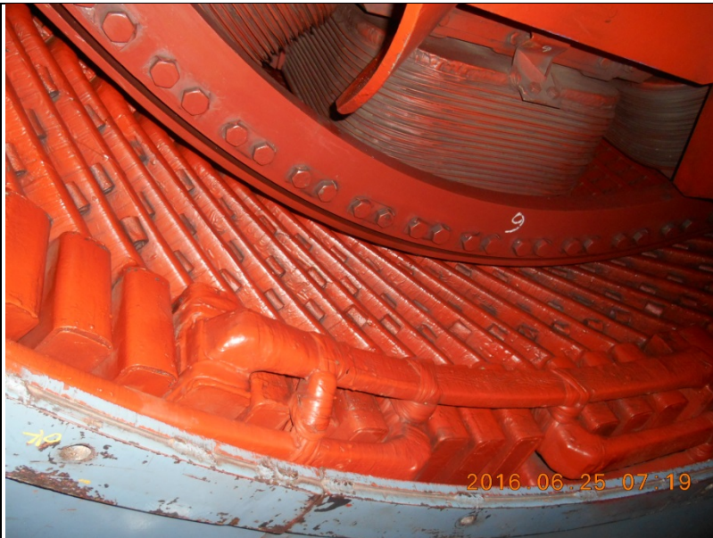
Fig. 5: Stator end turn and coil extension condition
