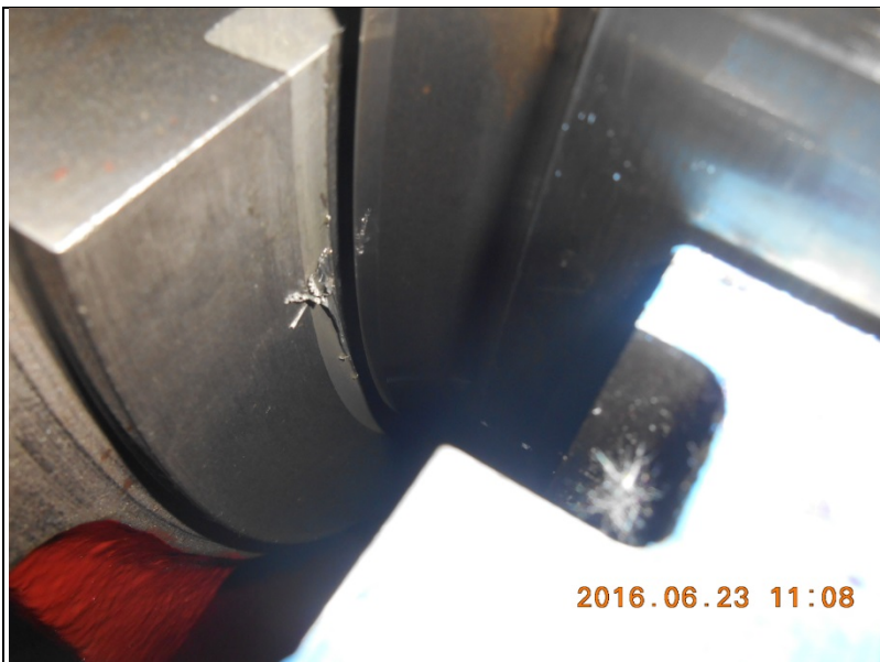
Fig. 23: Bearing damage found on outboard side
