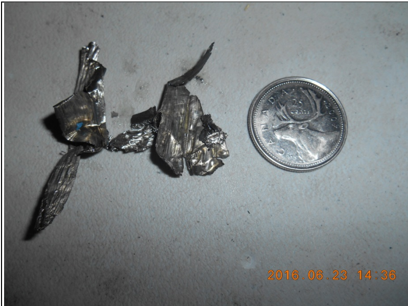
Fig. 22: Total babbitt from the bearing pedestal sump
