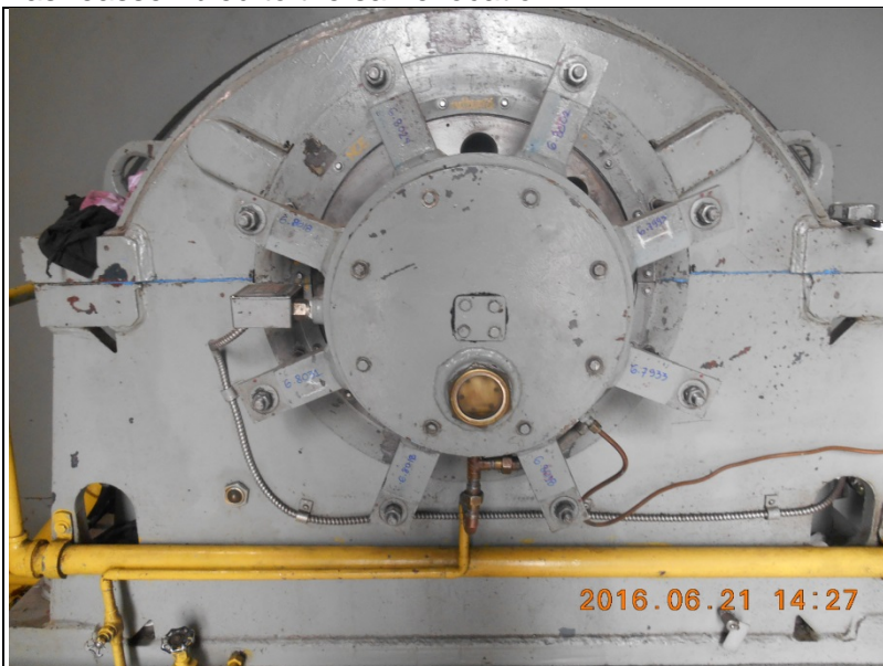
Fig. 26: Thrust Bearing offset measurements
